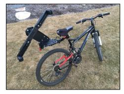
4. Insert bow. Check all fasteners for tightness and general setup for adequate bow and rider clearance. Happy Trails!
